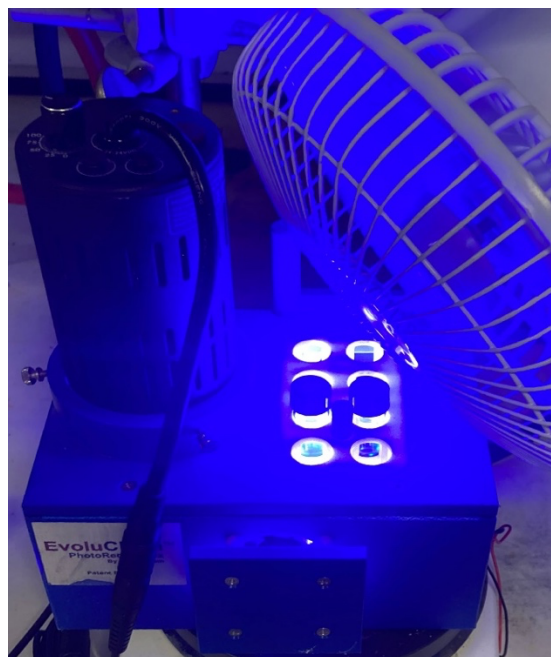
Fig. S2. Kessil PR160L 440 nm LED in an EvoluChem™ PhotoRedOx box.
