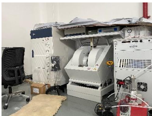
Figure S18. Set-up for electron paramagnetic resonance (EPR) studies
