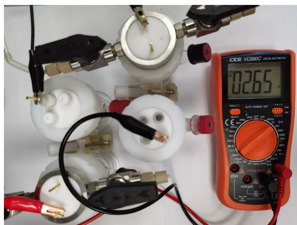
Figure S39. Photographic image of two Zn-CO 2 batteries connected in series, which exhibit an OCV of 2.65 V measured by a multimeter.
