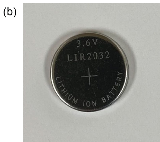
Figure S23. Digital pictures of the Swagelok cell and the coin cell setups used for electrochemical studies in this work. Swagelok cell enabled tests in three-electrode configuration and typically accommodates ~2 ml of electrolyte. Coin cell setup uses a relatively small amount of electrolyte (50 microliters).
