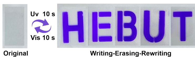
Figure S18. (a) UV-induced writing / rewriting and Vis-induced erasing behavior on a P1 film (about 3 cm × 4 cm).
