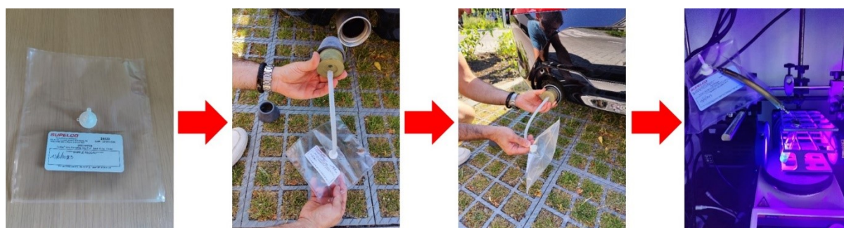
Figure S 6. The collection procedure of exhaust gasses.
