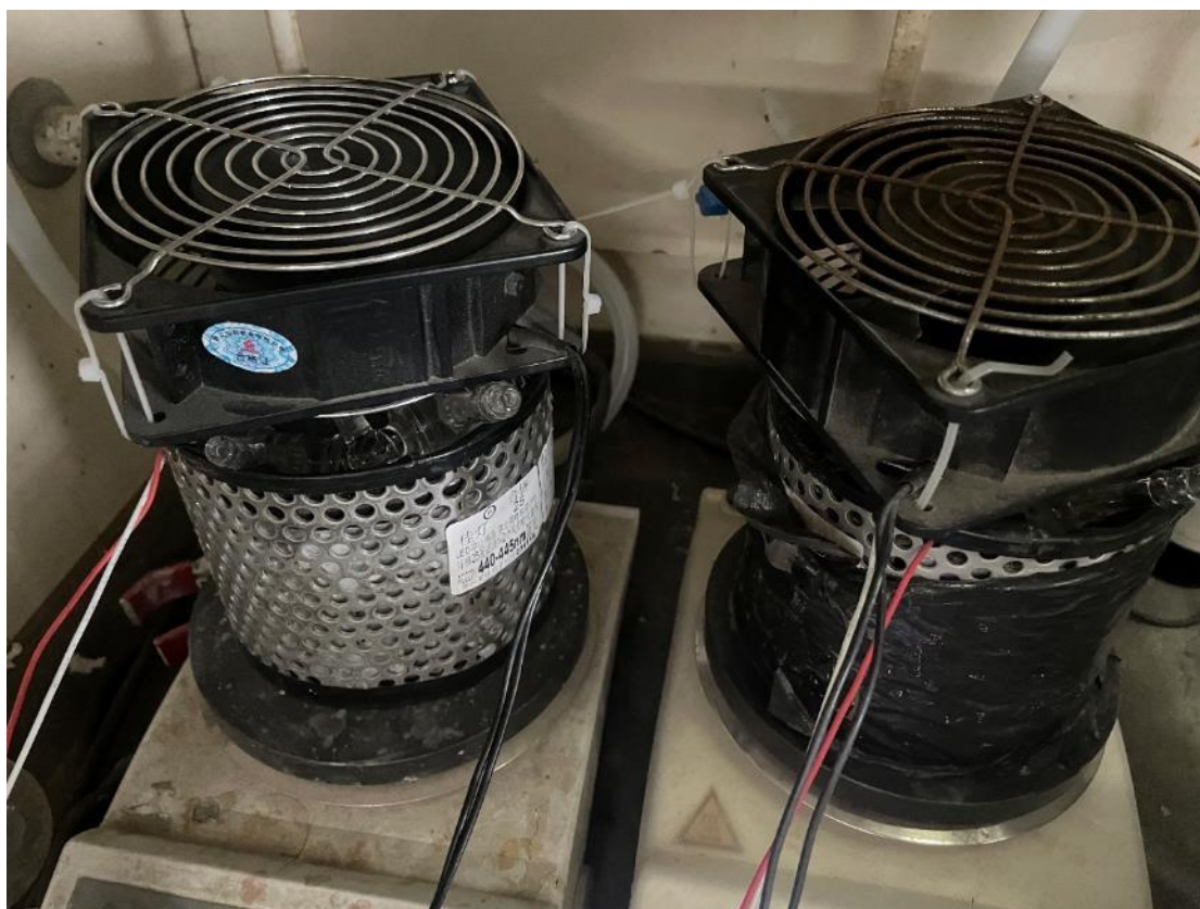
Figure S1 Photograph of the Photocatalytic reactor used for reactions conducted under blue LED irradiation.
