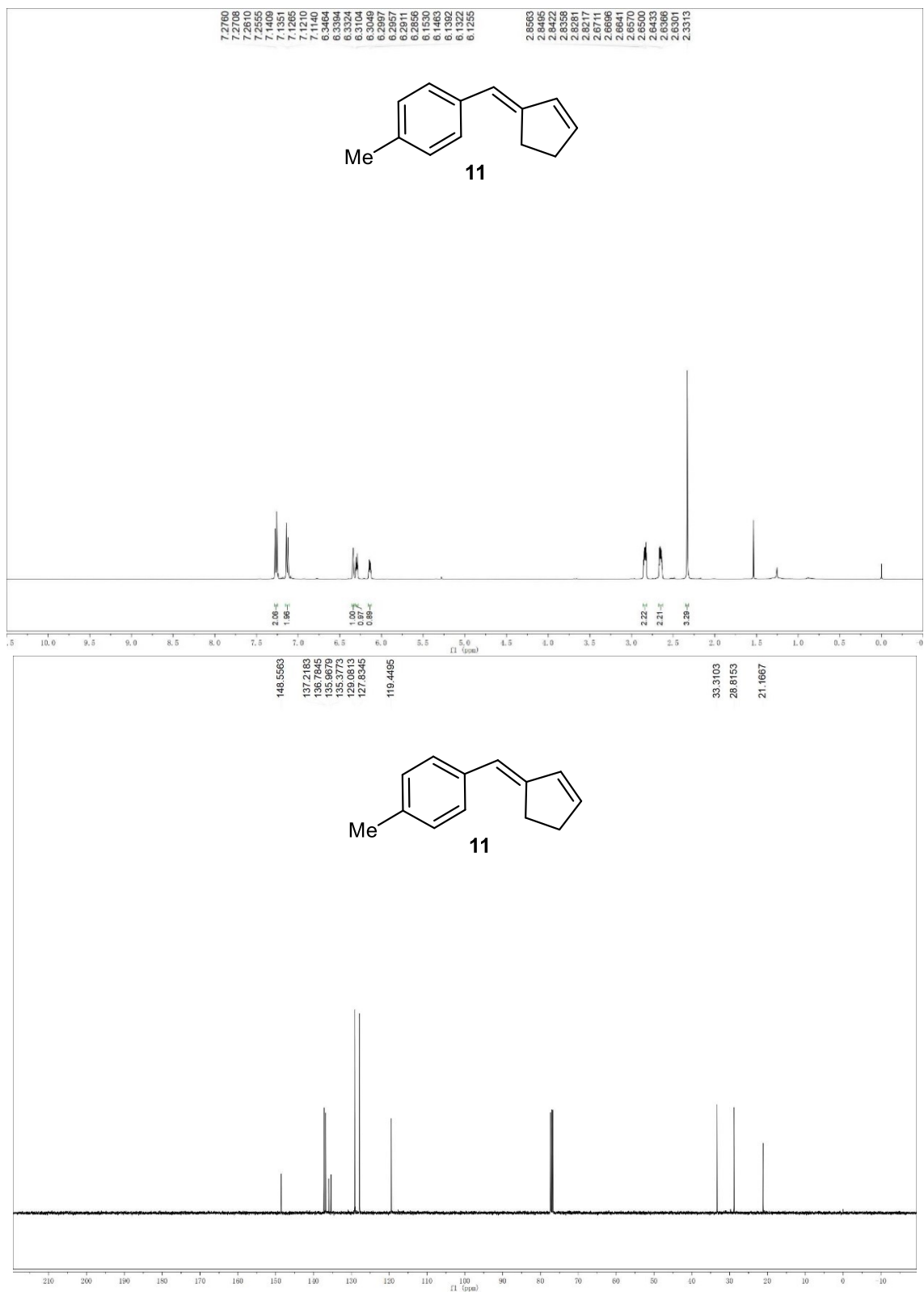
Figure S60. 1 H (400 MHz, CDCl 3 ) and 13 C (100 MHz, CDCl 3 ) NMR spectra for compound 11
