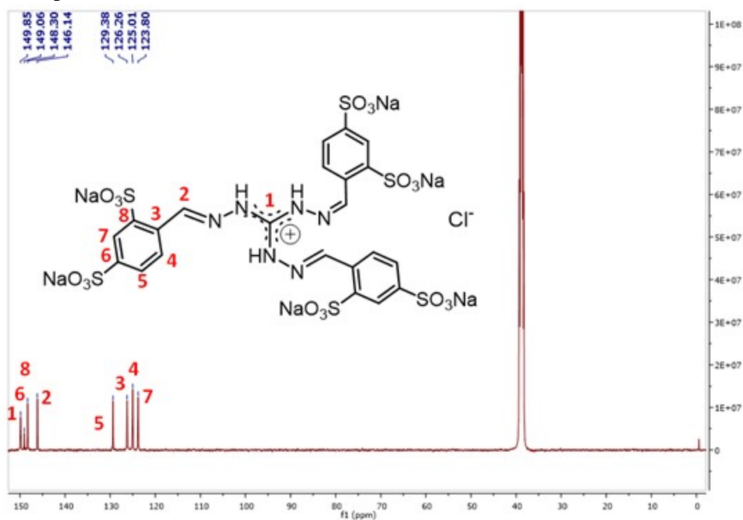
Figure S8: ^{13}\text{C} NMR spectrum of AD-1 recorded in \text{DMSO-}d_6
