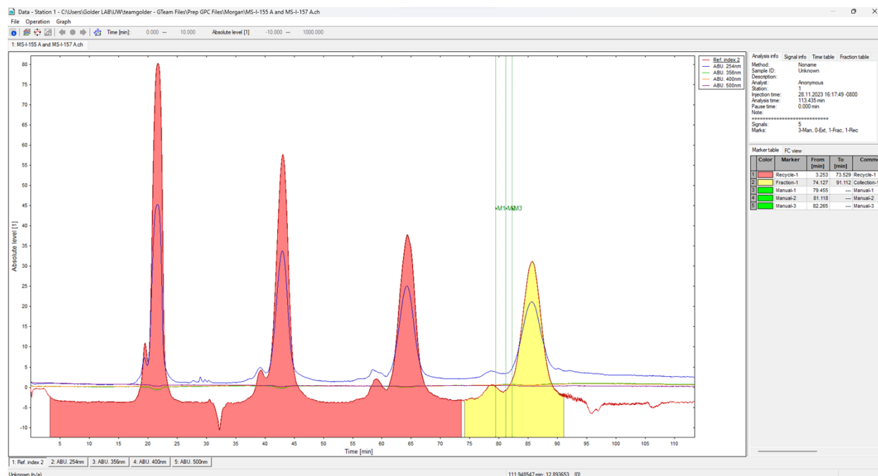
Figure S1. Preparative GPC trace of TFM-PS . The product was collected on the fourth cycle to allow appropriate separation of polymer peaks.
