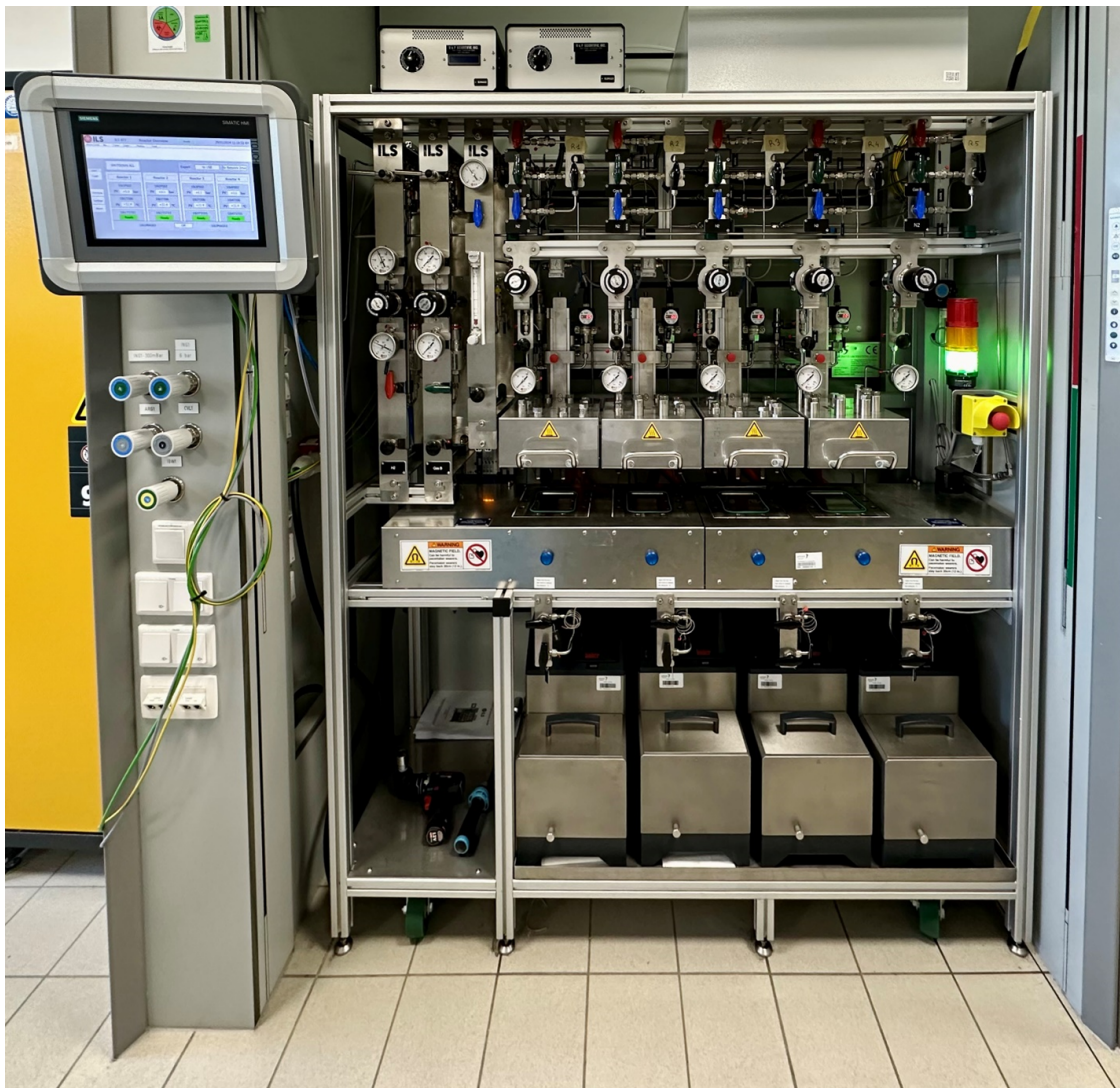
Figure S1: Parallel reactor system used in this work (Integrated Lab Solutions, Berlin, Germany).
