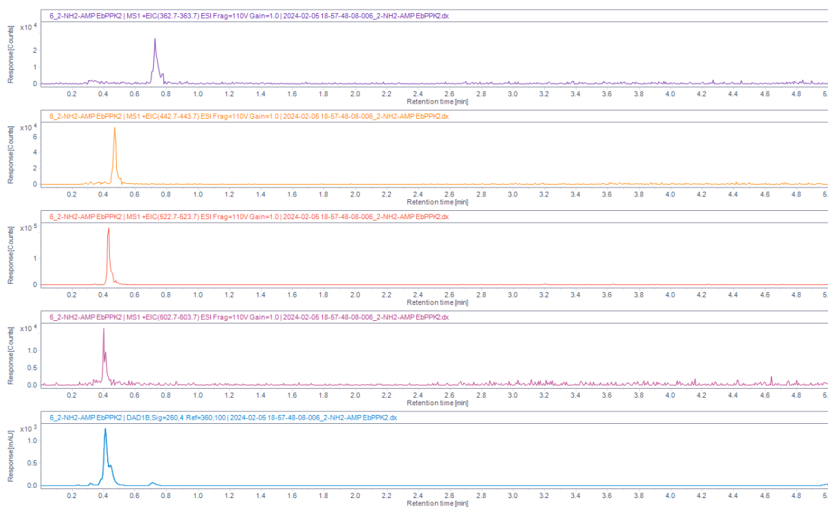
Figure S38: LC-DAD-Q-MS analysis of the EbPPK2 reaction starting from 4a . EIC for 4a , 4b , 4c , 4d and the UV trace at 260 nm.
