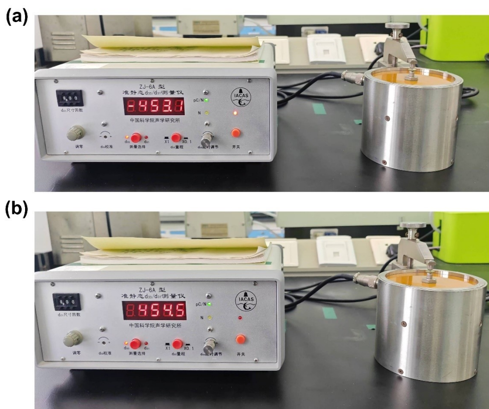
Fig. S6 Piezoelectric d_{33} data of polycrystalline pellet of 1 in reverse (a) and forward (b) connection.
