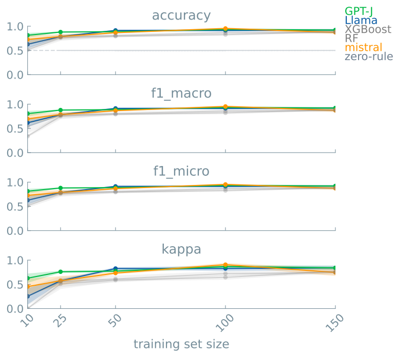
Figure 56. Learning curve analyses of binary classification of the melting point using different models. Three LLMs (GPT-J, Llama, and Mistral) and two traditional ML models (XGBoost and random forest (RF)) were validated on predicting the binary class of the melting point of TAGs. We used 50% as a random guess accuracy (dashed line), representing the zero rule baseline. Three runs were performed for each model to get the metric's average and standard deviation. SMILES of the TAGs were used as the input for the LLMs. Morgan Fingerprints of the TAGs were used as the input for the traditional ML models. The fine-tuned model reached the maximum accuracy of 92% (training set size of 150 and 25 epochs).
