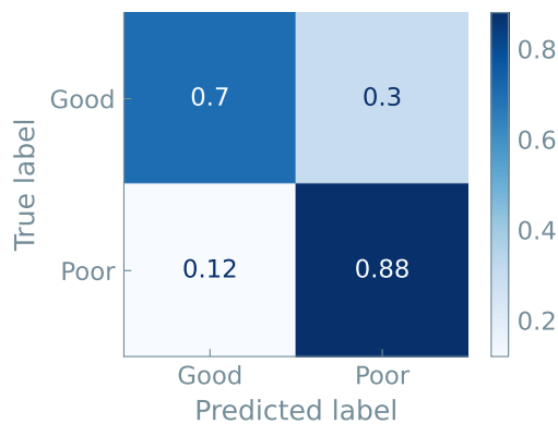
Figure 67. Normalized confusion matrix of models predicting the performance of the nickel catalyst. The confusion matrix contains the combined predictions of 10 individual training/test runs (GPT-J). A balanced dataset of 100 data points was used for training, number of epochs and the learning rate were set to 20 and 0.0003, respectively. The average accuracy over 10 unique models was 78.5%.
