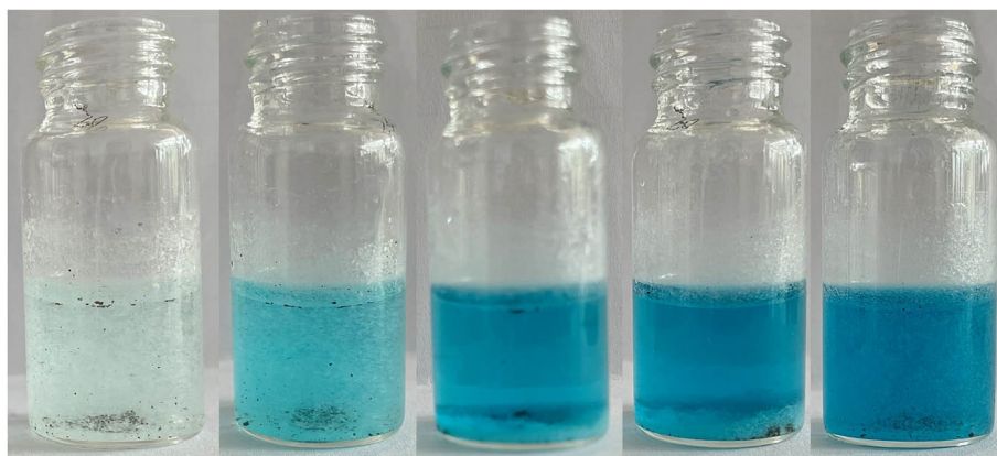
Figure S37. Color of the solution changes to blue (oxTMB) after the cascade catalytic reaction of GOx&HRP@HOF-PTBA.
