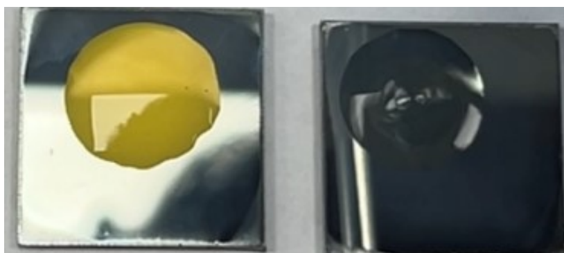
Figure S12. Surface images of the perovskite films before modification (left) and after modification (right) taken 5 seconds after dropping a water droplet simultaneously.
