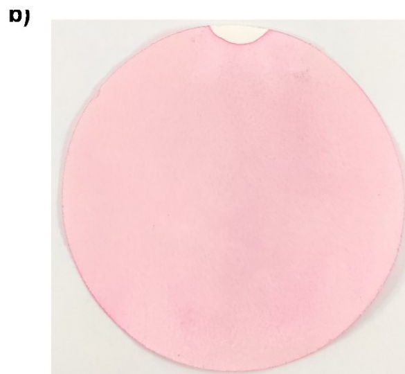
Figure S7. Photos of DASA-2@PMMA/LA capsules (a) and the filter paper loaded with DASA-2@PMMA/LA capsules (b) using the spray coating method.
