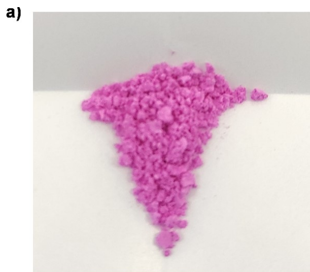
Figure S7. Photos of DASA-2@PMMA/LA capsules (a) and the filter paper loaded with DASA-2@PMMA/LA capsules (b) using the spray coating method.
