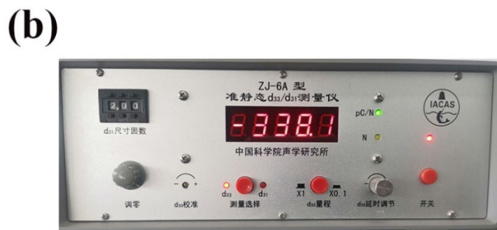
Figure S6 Piezoelectric d_{33} data of 1 (polycrystalline films): (a) forward in up connection, (b) reverse in down connection.
