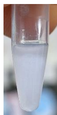
Figure S10: BSA protein is coagulated in the presence of Zn(OAc) 2 (400 μM)
