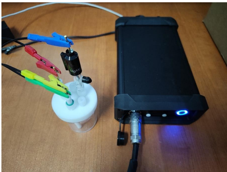
Figure S7. Cyclic voltammetry (CV) setup.
