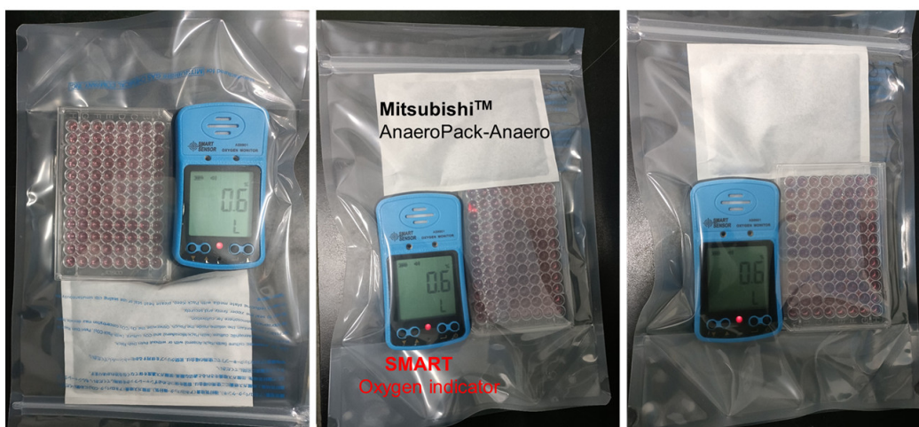
Fig. S36 The photograph of mimicking hypoxic environment via Mitsubishi™ device for 4 h and measuring the content of O 2 using the oxygen indicator. Results are presented through three repeated measurements.
