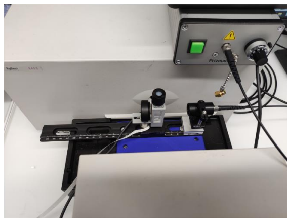
Figure S13. A) Irradiation module with magnetic stirring and exchangeable LED modules. B) In-house built irradiation setup with collimated light beam (780 nm) with magnetic stirring and coupled to optical power meter. C) Setup from (B) mounted inside a UV-vis spectrometer.
