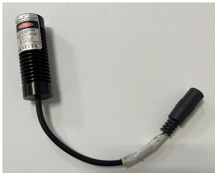
Figure S3. Image of the external laser source of 405 nm
