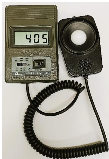
Figure S4. Image of lux meter LX-101 (taken under the lab lights)
