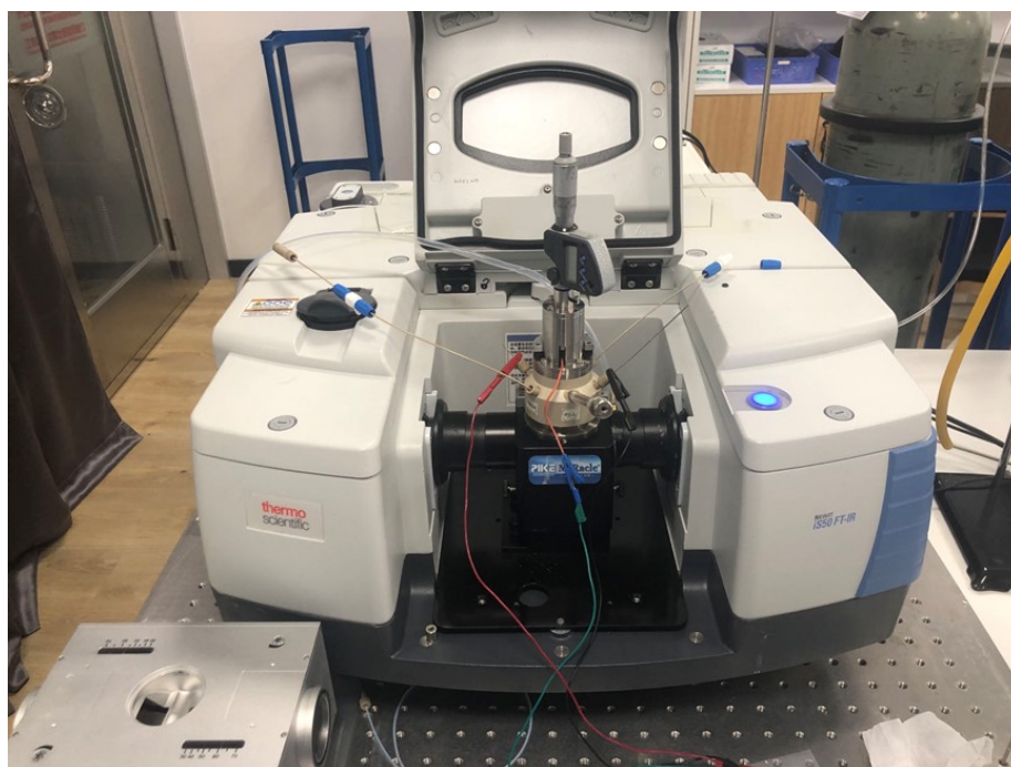
Fig. S21 In situ Fourier transform infrared spectroscopy (FT-IR) test equipment for spectroelectrochemical experiments.
