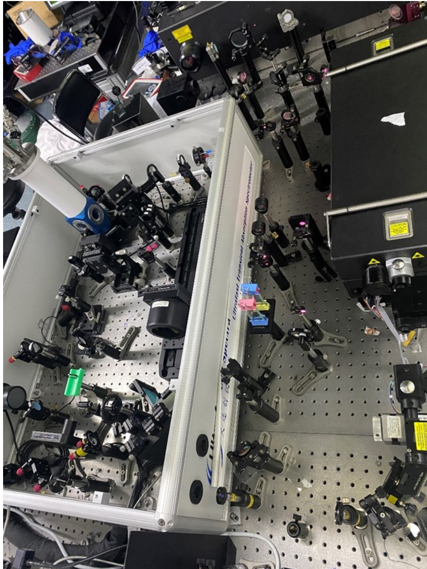
Fig. S5 Femtosecond pump-probe transient absorption measurements system.
