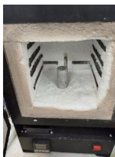
Figure S1. Muffle furnace “satellite” Russia. Maximum heating temperature: 1200 °C.
