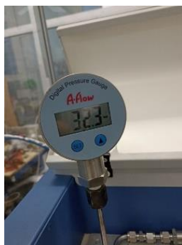
Figure S2. Photo of a steel reactor pressure gauge heated to 500 °C.
