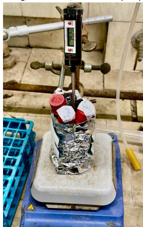
Figure S3. organoindium reaction set-up.
