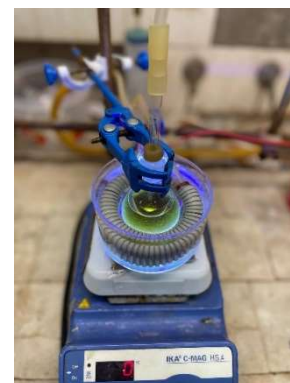
Figure S11. Gram scale reaction photocatalytic set-up
