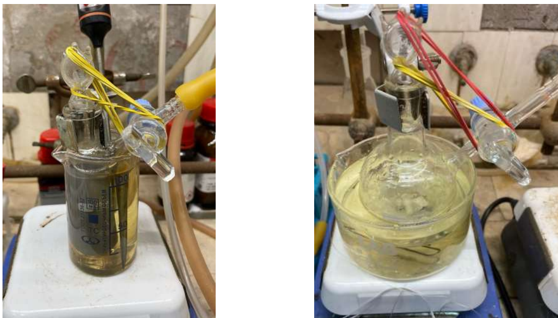
Figure S5. Preparation of reagent 2c-Cl with indium precipitation in the form of powder (left) or nuggets (right).
