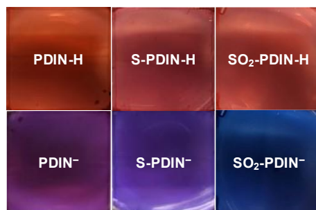
Figure S16. Images of PDIN-H (left), S-PDIN-H (centre) and SO 2 -PDIN-H (right) films before and after exposure to n-butylamine. Top images are prior to amine exposure, bottom images are after exposure. Films are spin-coated from MeTHF (S-PDIN-H, SO 2 -PDIN-H) or butylamine (PDIN-H) on a flexible PET substrate with an anti-static coating to enable thick films.
