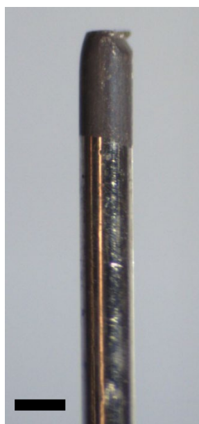
Supplementary Fig 5. Micrograph of Ag/AgCl electrode. The image shows a chamfer on the tip of the electrode which may have impacted the size of lipid bilayers formed. Scale bar = 500 \mu m.
