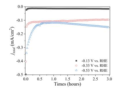
Figure S1 – Chronoamperometries Curves using the prepared electrode applying different potentials. 3 hours.
