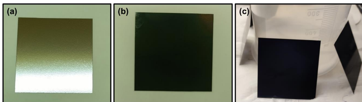
Figure S2. Digital image of thin Si wafers (a) planar, (b) 90s etched SiNW, (c) prepared 4.5 \times 4.5 \text{cm}^2 black Si wafers for solar cell fabrication.
