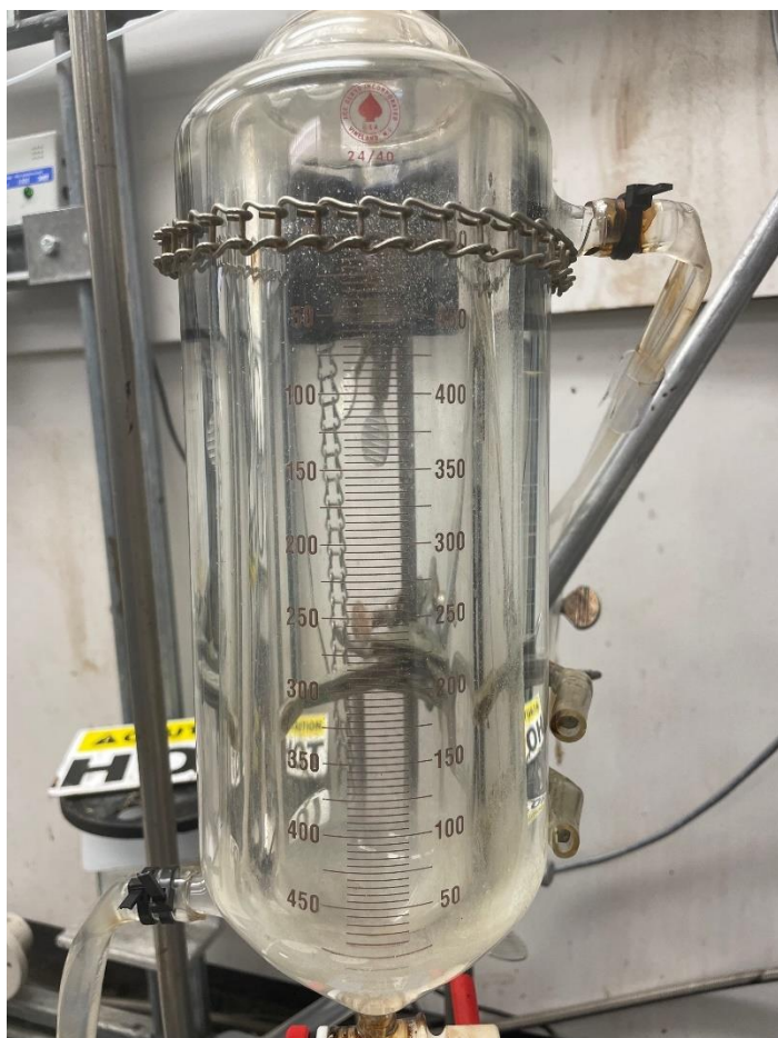
Figure S2. Image of the jacketed glass funnel used in this work.
