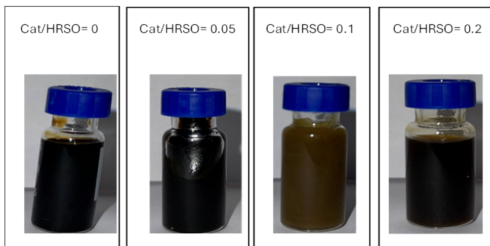
Figure S12: Appearance of oil/wax products obtained by varying 5 wt% Pt/C catalyst/HRSO mass ratios at 400 °C for 1 h reaction time
