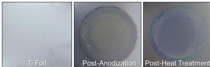
Figure S4. Pictures of  $\text{TiO}_2$  NTs photoelectrode from resulting anodization and annealing.
