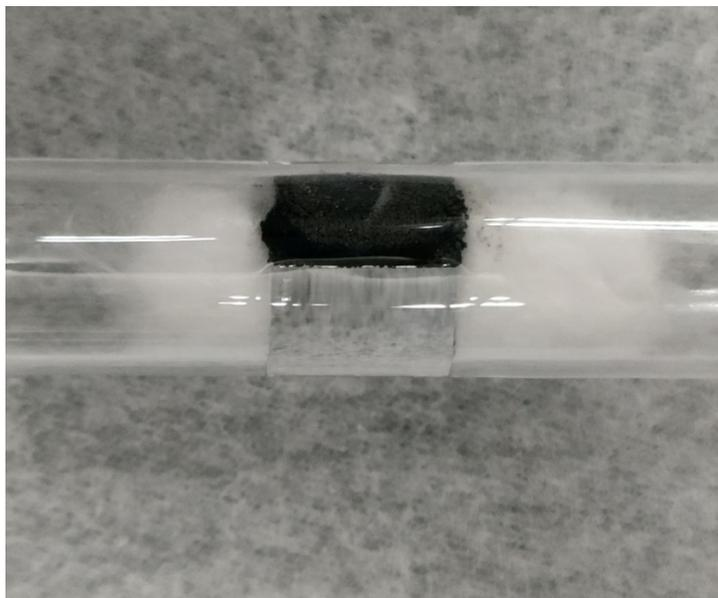
**Figure S1** Photograph of the 1-mm-gap reactor filled with 35 mg of  $\text{Co}_5\text{Ni}_{95}\text{@SiO}_2$  catalyst.
