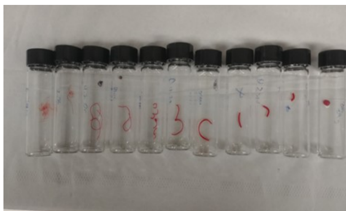
Fig. S7. PMI-SA-2.5 extruded into 0.5 M \text{CaCl}_2 from different nozzle diameters. From left to right 0.191 mm, 0.241 mm, 0.318 mm, 0.394 mm, 0.495 mm, 0.584 mm, 0.838 mm, 1.194 mm, 1.372 mm, 1.6 mm, and bulk blob. Plot of the ratio between the TON with the 27G (0.191 mm) and 20G (0.584 mm) samples at varying SA loadings. PMI-SA-1 and PMI-SA-2 were prepared with SA loading between 1 wt% and 4 wt% and each ink was extruded through a 27G nozzle (0.191 mm) or a 20G nozzle (0.584 mm). For instance, PMI-SA-1 shows a ratio of 1 at 1wt% loading, indicating that the diffusivity of SA is high enough that the HER is not affected by a reduction of gel diameter. However, the ratio increases with higher SA loading indicating that slower diffusion enhances the effect of decreasing gel diameter.
