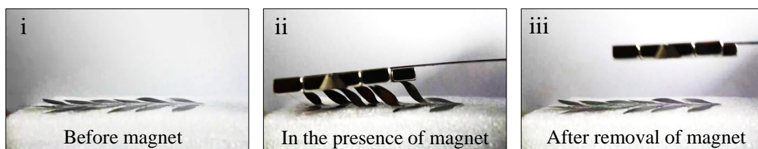
Figure S12: (i) The leaflets made up of the composite film in the absence of the magnetic field, (ii) the bending state of the leaflets in the presence of the external magnetic field, (iii) the leaflets return to their original state after removal of the external magnetic field.
