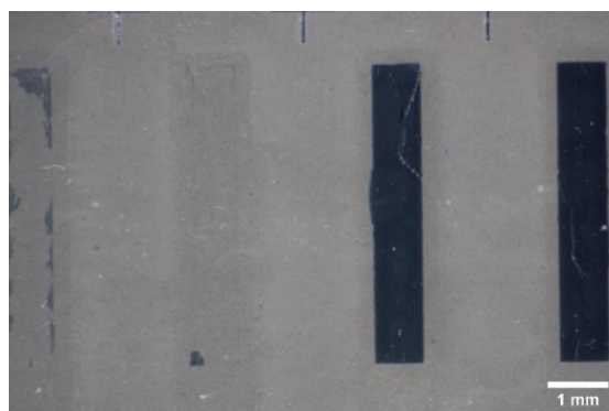
Fig. S2. Leftover bottom layer PEDOT:PSS after actuators (design A in Fig. S1 ) with different PEDOT:PSS thicknesses are peeled off. Left to right: 1 printing pass, 2 printing passes, 3 printing passes, and 4 printing passes.
