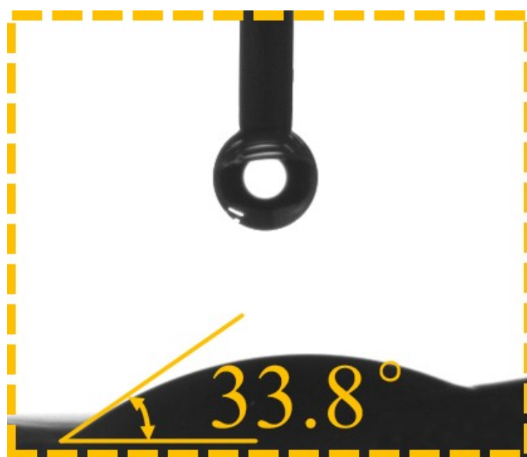
Fig.S3. Contact angle measurement of NiCo-MOF/GO/CNTs-II
