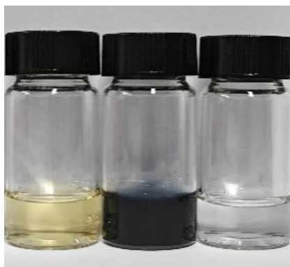
Fig. S4 Photograph showing the color changes in pAMPS-Cl during the iodometric titration.
