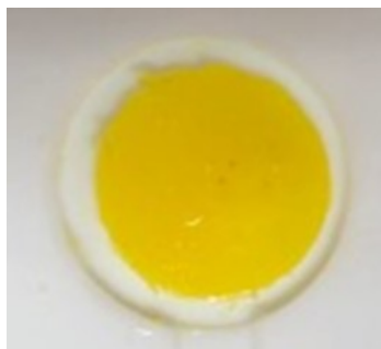
Figure S20. Hydrogel sensor against a control model sweat solution without urea showing no colorimetric response.
