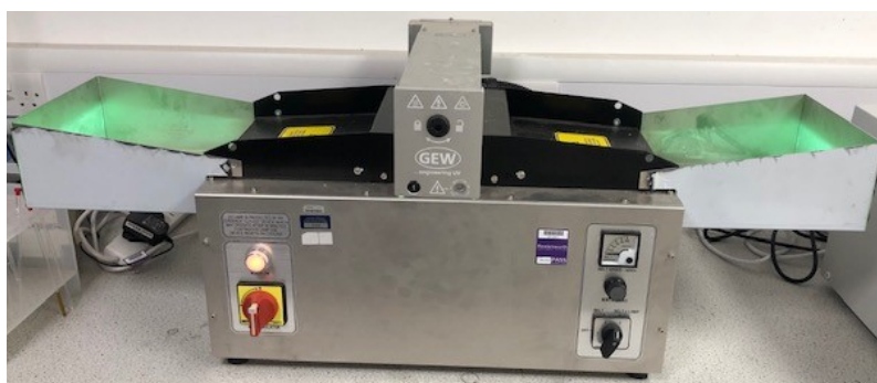
Figure S1. The VCP-15-LAB benchtop UV curing conveyor belt used for the hydrogel synthesis.
