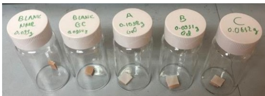
Figure S22. PEG700-DA/PEG1000 (39.5 vol%) sensor gels ( \times 3 replicates) on the top of Bioskin ® specimens for leachable studies.
