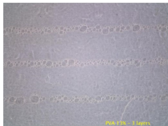
Figure S8. Bubble formation of screen-printed PVA. Photographs and 3D profile of 13% PVA printed on PC without surfactant (top). Micrographs of meander structures printed on PC using 13% PVA.
