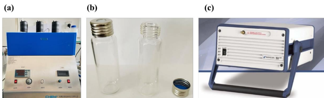
Fig.S8 (a)customized photoreactor;(b)customized reaction bulb;(c)Micro GC
