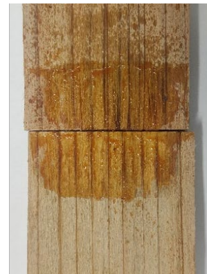
Soak in boiling DI water for 4 h → soak in DI water at 60 °C for 20 h → soak in boiling DI water for 4 h → soak in DI water at 20 °C for 10 min
