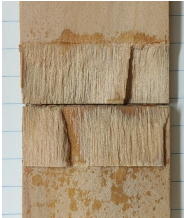
Figure S1. Cypress fractured by shear forces.
