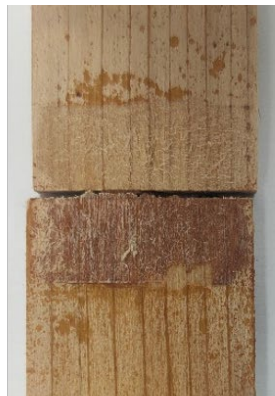
Soak in DI water at 60 °C for 3 h → soak in DI water at 20 °C for 10 min
