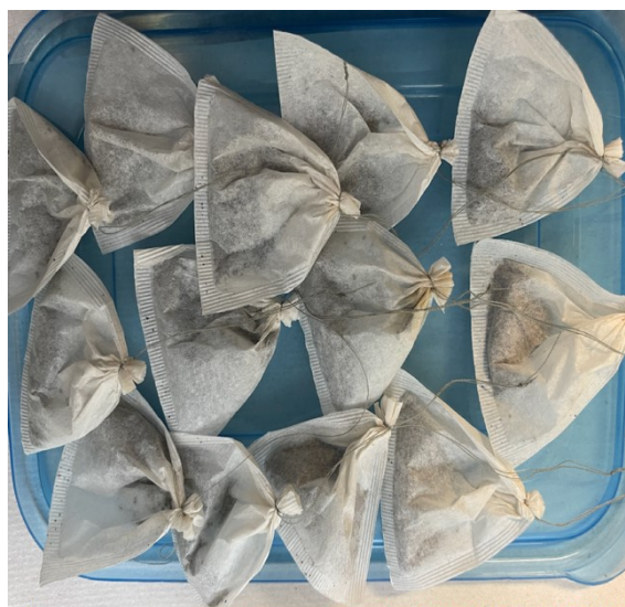
Fig. S5 Performing water retention studies using tea bag method
