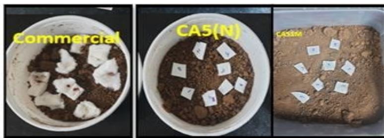
Fig.1. Experimental setup for soil burial test
