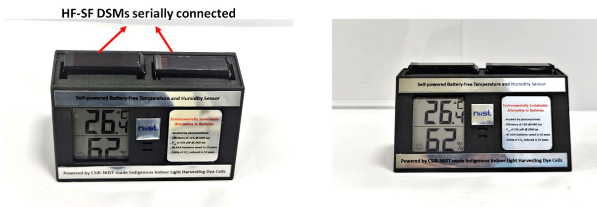
Figure S17. Indoor weather monitoring unit (temperature and humidity sensor) powered by serially interconnected HF-SF DSMs using co-sensitized D35:XY1b dyes and [\text{Cu}^{(\text{II})}(\text{dmp})_2] electrolyte.
