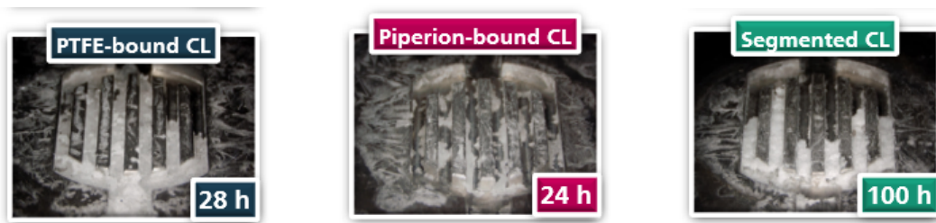
Figure S8: Photograph of the parallel flow fields directly after disassembling the zero-gap cells after long-term electrolysis
