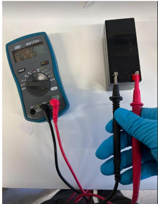
**Figure S1.** The voltage of the lead-acid battery **a)** before and **b)** after discharging process.
