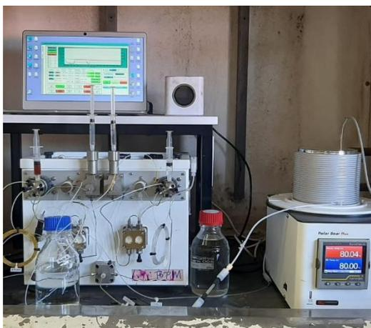
Figure 3: Protection (potassium hydroxide) setup using Uniqsis Binary Pump
