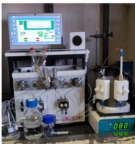
Figure 1: Phenolic allylation (potassium carbonate approach) setup using Uniqsis Binary Pump
