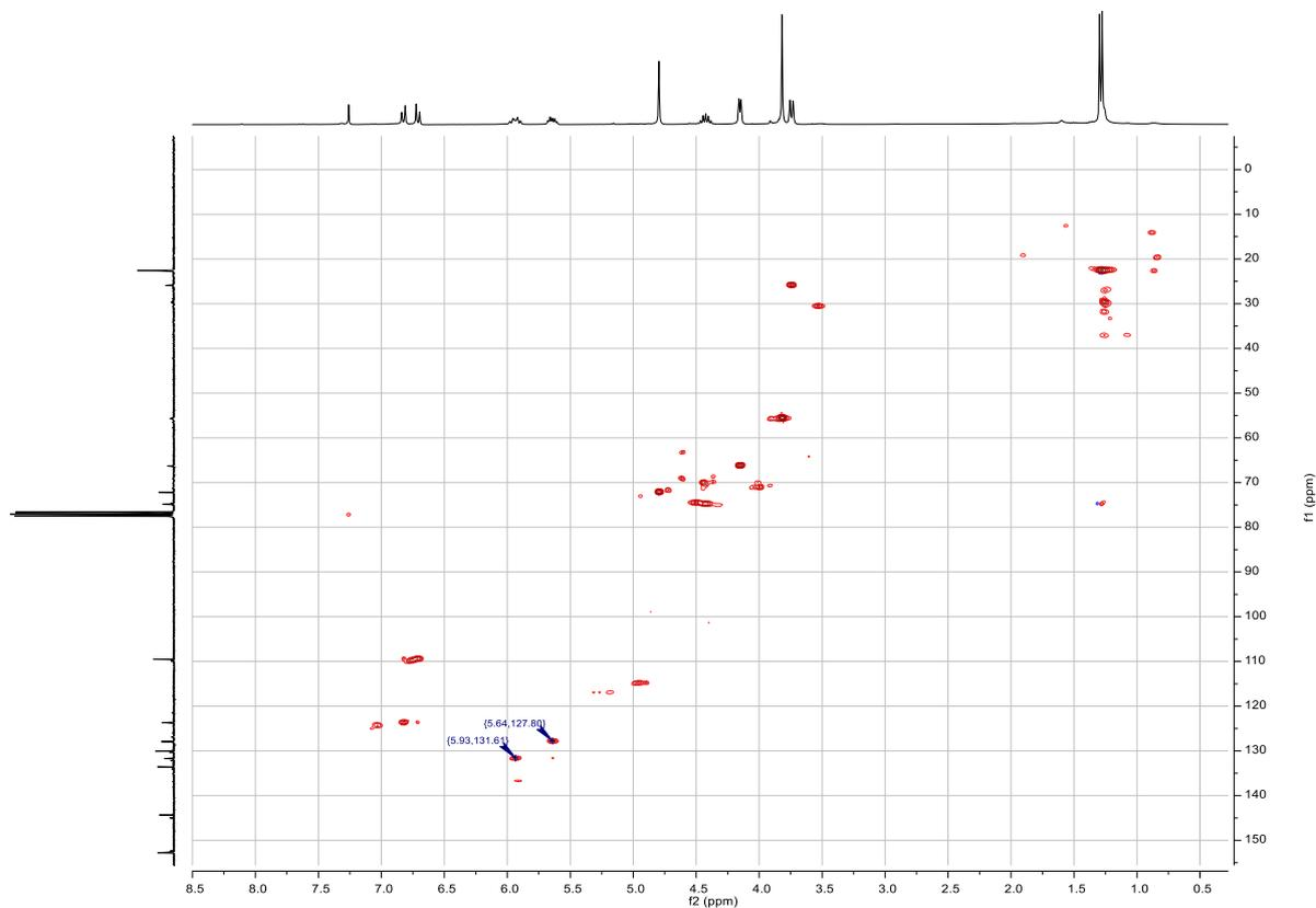
NMR 20: HSQC NMR spectrum for (Z)-7-isopropoxy-8-methoxy-3,6-dihydro-1H-benzo[c]oxocine 1
