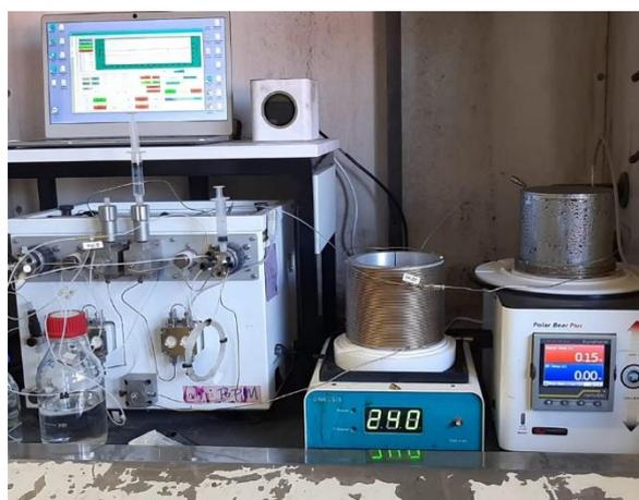
Figure 2: Claisen rearrangement setup using Uniqsis Binary Pump
