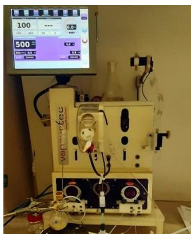
Figure 7: Second allylation (sodium hydride approach using recycling approach) setup using Vapourtec peristaltic pumps
