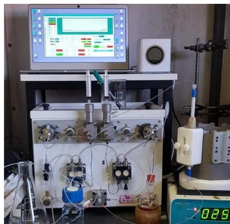
Figure 4: Reduction (polymer supported sodium borohydride approach) using Uniqsis Binary Pump
