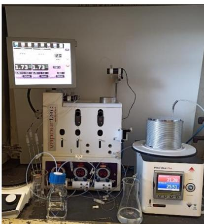
Figure 5: Reduction (sodium borohydride solution approach) using Vapourtec peristaltic pumps
