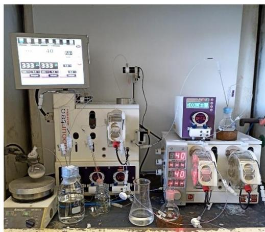
Figure 6: Second allylation (sodium hydride approach using standalone) using Vapourtec peristaltic pumps
