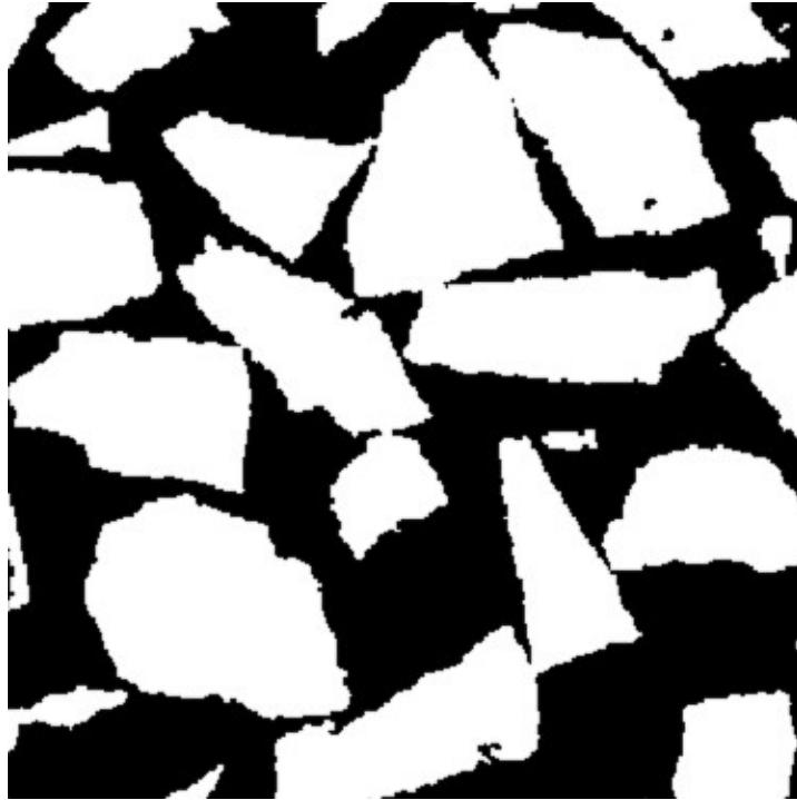
Figure S8: Example visual slice of the CZA packed bed reactor processed using MicroCT and MATBOX postprocessing.
