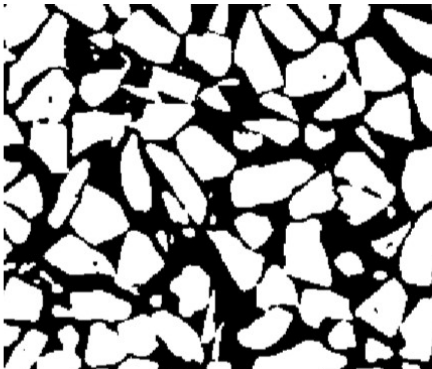
Figure S15: Example visual slice of the mixed packed bed reactor processed using MicroCT and MATBOX postprocessing.
